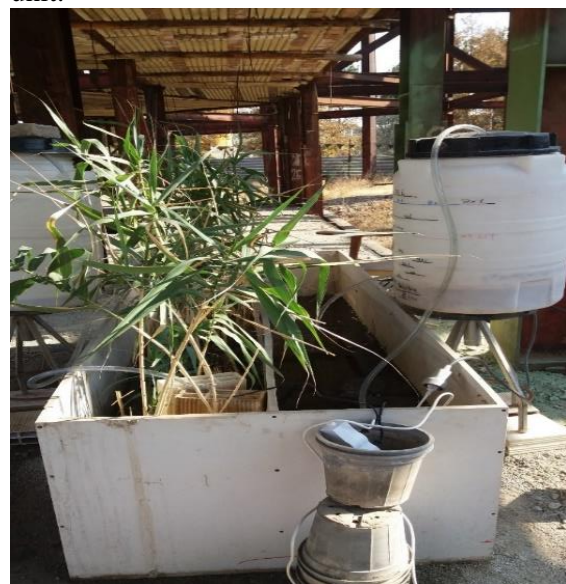
Fig.3. A laboratory-scale pilot (the second pilot) containing two units (1. planted unit, 2. Control unit)
