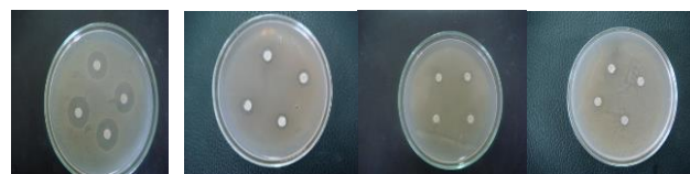
Figure 2. Inhibitory halo of paper disc impregnated with thyme, mint and neem extracts, and copperoxychloride on Pectobacterium carotovorum subsp. carotovorum (left to right)
